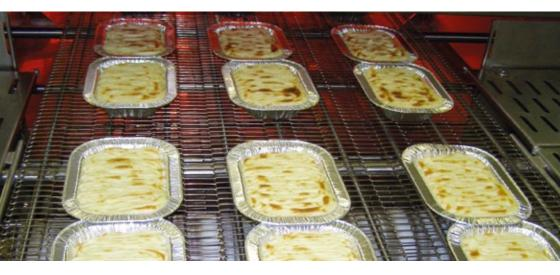
WMH inline industrial grilling units are designed to add colour to the top of ready meals and convenience foods without increasing the core temperature of the product. The infrared heater panels provide even heat across the width of the grill and the quick reaction time enables panels to be at optimum operating temperature almost instantaneously.
