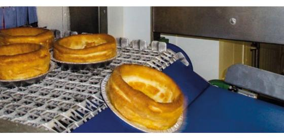
WMH freezer loading systems integrate with your assembly lines or ovens and will gently collate or lane products across the belt to ensure your line runs efficiently with optimum product loading to achieve the maximum throughput for your production line.
