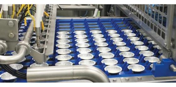
WMH hygienic multi-lane depositing systems are designed for depositing hot or cold liquids and sauces at high throughputs and with great repeatable accuracy. Our depositors can be supplied as stand-alone mobile units or can be fully integrated into the production line.
